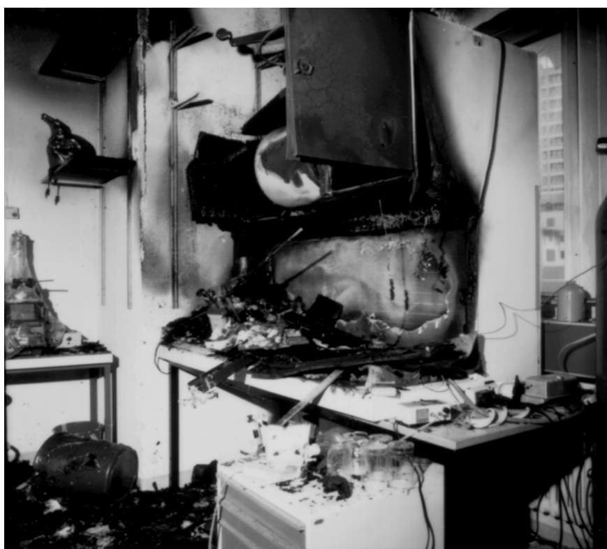
Fig. 3.1: Result of a laboratory fire due to inappropriate handling of flammable chemicals
